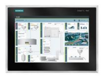
SIMATIC HMI TP1200 Comfort INOX Stainless steel front, Glass pane, capacitive touch, Degree of protection front IP69K, 12" widescreen TFT display, PROFINET interface, MPI/PROFIBUS DP interface, 12 MB configuration memory, Windows CE 6.0, (Microsoft Support included Security updates discontinued) configurable from WinCC Comfort V15
